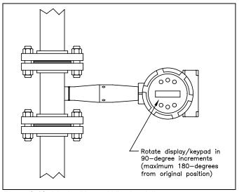
Figure 2-12. Display/Keypad Viewing Adjustment
