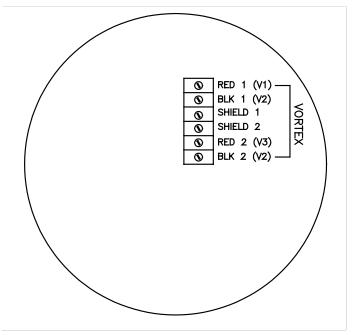
Figure 2-17. Junction Box Sensor Connections
