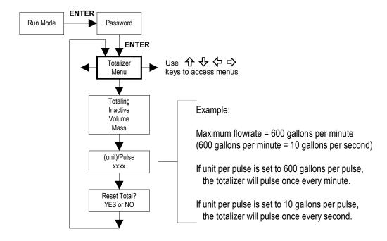
Use the Totalizer Menu to configure and monitor the totalizer. The totalizer output is a 50 millisecond (.05 second) positive pulse (relay closed for 50 milliseconds). The totalizer cannot operate faster than one pulse every 100 millisecond (.1 second). A good rule to follow is to set the unit per pulse value equal to the maximum flow in the same units per second. This will limit the pulse to no faster than one pulse every second.
