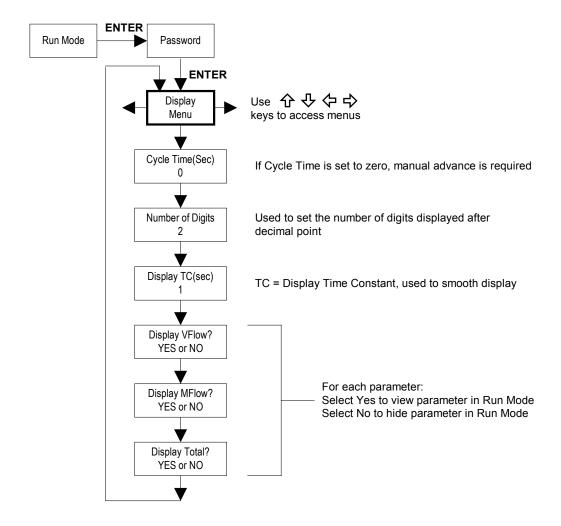
Use the Display Menu to set the cycle time for automatic screen sequencing used in the Run Mode, change the precision of displayed values, smooth the values or enable or disable each item displayed in the Run Mode screens.
