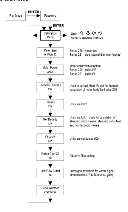
The Calibration Menu contains the calibration coefficients for the flow meter. These values should by changed only by properly trained personnel. The Vortex Coef Ck and Low Flow Cutoff are set at the factory. Consult the factory for help with these settings if the meter is showing erratic flow rate. The units of measurement used in the Calibration Menu are preset and are as follows: Density = lbm/ft³, Reference Density = lbm/ft³, Viscosity = centipoise.
