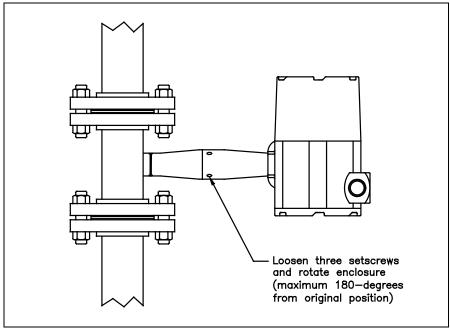
Figure 2-13. Enclosure Viewing Adjustment
