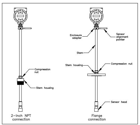
Figure 2-7. Flow Meter with Compression Type Fitting
