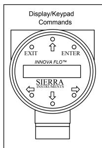
From the Run Mode, theENTER key allows access to the Setup Menus (through a password screen). Within the Setup Menus, pressing ENTER activates the current field. To set new parameters, press the ENTER key until an underline cursor appears. Use the ① 中中 keys to select new parameters. Press ENTER to continue. (If change is not alllowed, ENTER has no effect.) All outputs are disabled when using the Setup Menus.
