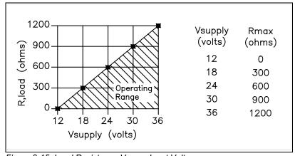
Figure 2-15. Load Resistance Versus Input Voltage
