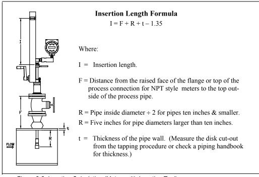
Figure 2-8. Insertion Calculation (Meters with Insertion Tool)
