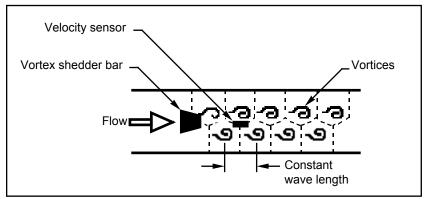
Figure 1-2. Measurement Principle of Vortex Flow Meters
