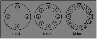
Figure 2-2. Flange Bolt Torquing Sequence
