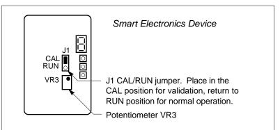
Figure 3-2. Electronics Validation Component Locations
