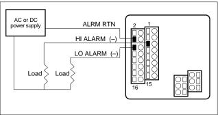
Figure 2-8. Isolated Alarm Output Connections
