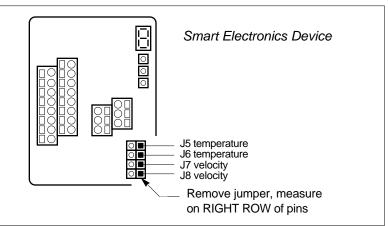
Figure 3-3. Sensor Validation Component Location
