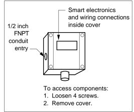
Figure 2-2. Wiring Access
