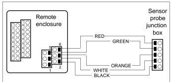
Figure 2-11. Sensor Junction Box to Remote Enclosure Connections
