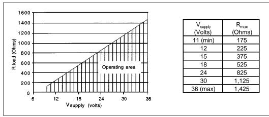
Figure 2-5. Load Resistance Versus Input Voltage
