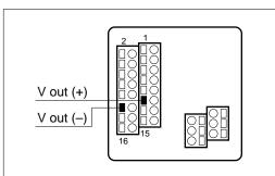
Figure 2-4. VDC Output Wiring Connections
