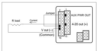
Figure 2-7. Non-isolated 4-20 mA Current Loop Connections
