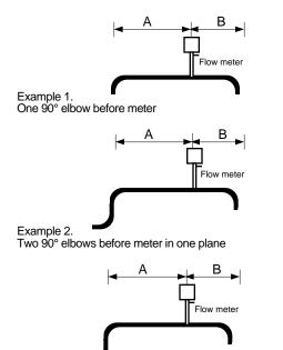
Example 3. Two 90° elbows before meter out of plane (if three 90° bends present, double recommended length)
