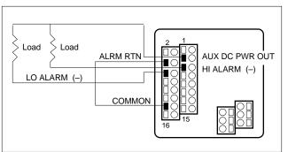
Figure 2-9. Non-isolated Alarm Output Connections
