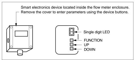
Figure 3-1. Display/Keypad Commands
