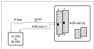
Figure 2-6. Isolated 4-20 mA Current Loop Connections
