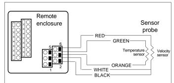
Figure 2-10. Remote Electronics Enclosure to Sensor Connections
