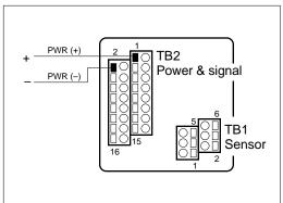
Figure 2-3. Input Power Connections
