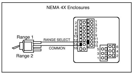
Figure 2-12. Range Selection Wiring
