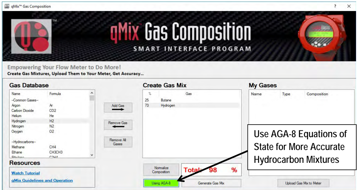
Figure 11. Use AGA-8 Equations of State for Higher Accuracy of Hydrocarbon Mixtures
