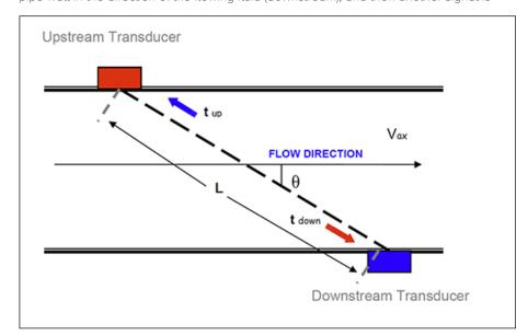
Figure 1: Transit-Time Ultrasonic Principle Of Operations
